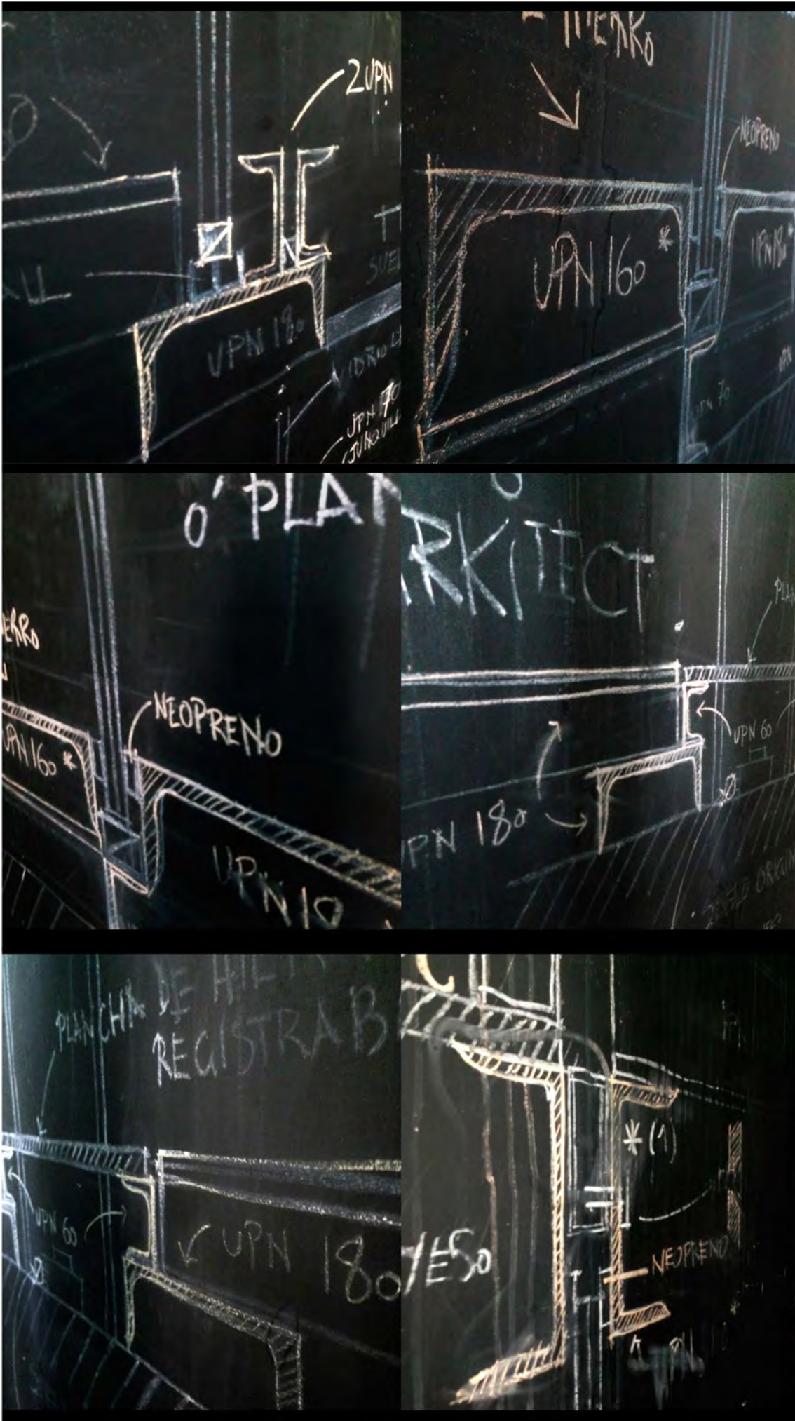
Left: Structural steel junction sketches on chalkboard, Nave 17c, Arturo Franco. Courtesy of Arturo Franco.
